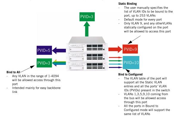
Figure 11.3 Multiple VLAN Per-port Binding Modes
